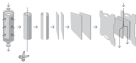
**Figure 2b:** Design for the cassette is derived from the capsule by cutting and creating two membrane stacks.
