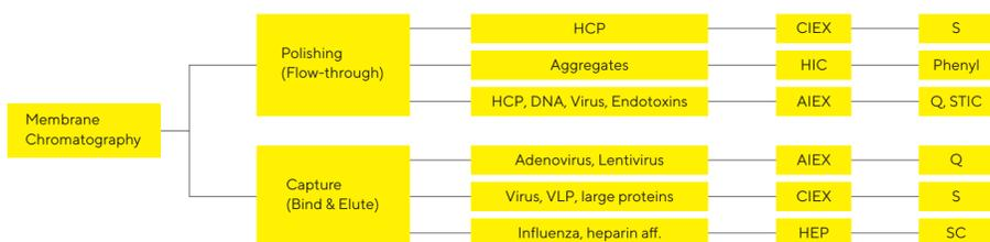
**Figure 1:** Typical modes of operations and applications for membrane adsorbers in the biopharmaceutical industry. Ligands: S = sulfonic acid for cation exchange (CIEX), Phenyl as hydrophobic interaction chromatography ligand (HIC), Q = quaternary ammonium, STIC = STIC PA primary amine (salt tolerant) for anion exchange (AIEX), SC = sulfated cellulose
