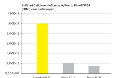
**Figure 8:** Evaluation of the recently developed SC displays ~5 to 7 × higher binding capacity of virus particles (VP)/mL, HAU/mL and ~6 × higher flow rate than conventional resin columns.<sup>3</sup> Comparison with influenza B/Phuket/3073/2013 showed even up to 23-fold higher binding capacity compared to resins.<sup>4</sup>
