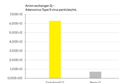
**Figure 7:** Comparison of Sartobind® Q binding capacity for Ad 5 displays about 9 times more binding capacity and ~100 times higher flow rate compared to a conventional resin.<sup>2</sup>
