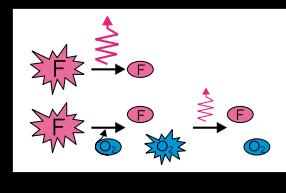
High oxygen saturation shows low emitted light intensity.
