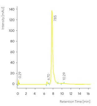
Figure 2: Elution of CIMmultus<sup>®</sup> C4 HLD fraction analyzed on CIMac™ pDNA-0.3 Analytical Column
