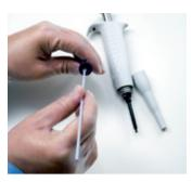
Proline® Plus pipettes have only three parts that need cleaning and maintenance.
