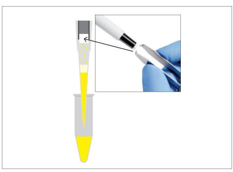
Tweezers for exchanging filters in pipettes are supplied with all pipettes excluding Tacta® and Mline®.
