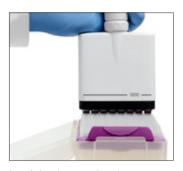
Load the tip onto the pipette carefully and take advantage of the Optiload tip loading mechanism.
