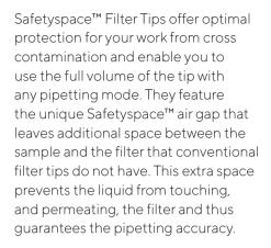
Safetyspace™ Filter tips are made of virgin polypropylene and are fitted with pure polyethylene filter barriers that effectively capture solid and liquid aerosol particles. The filter is made without self-sealing additives to avoid any interference with the sample or results. In addition to protecting your samples, the filter protects your pipette and prolongs its the maintenance interval.
