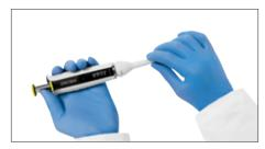
Unscrew the tip ejector collar counter clockwise and remove it. Remove the Safe-Cone Filter if fitted.
