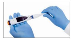
Unscrew the tip ejector collar counter clockwise and remove it. Remove the Safe-Cone Filter if fitted.
