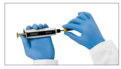
Unscrew the tip cone holder counter clockwise and carefully remove it along with the tip cone.
