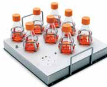
SENSOLUX® A shaker platform equipped with optical sensors for cell cultivation; in combination with single-use Erlenmeyer flasks, permits non-invasive measurement of the pH and dissolved oxygen values in incubation shakers
