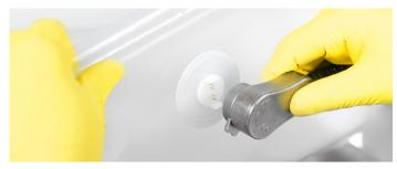
Figure 1: Viable Biomass Sensor (BioPAT® Viamass) Integrated in the Flexsafe® RM Bag - Connection to the Hardware Component.
