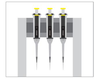
**Do use a pipette stand for storage** Use pipette stand to keep pipettes in a vertical position in order to avoid contamination, and to allow easy tracking of the pipette's location
