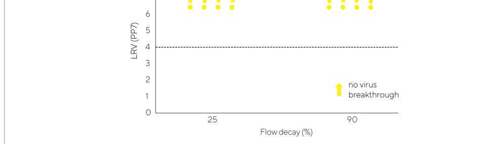
PP7 retention is independent of the level of flow decay, with absolute retention of >  $6 \log_{10}$  (without virus breakthrough).
