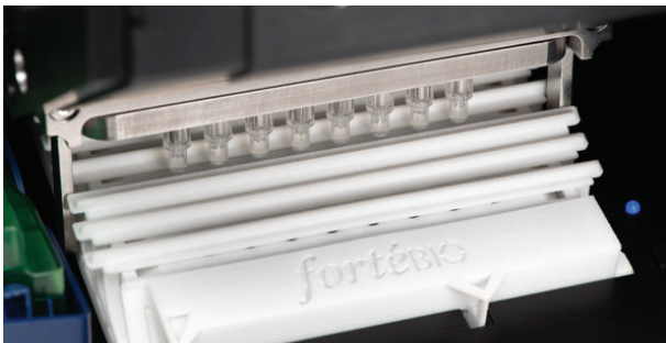
Figure 1: One column flap of the evaporation cover is opened to allow for the biosensors to dip into the sample wells..
