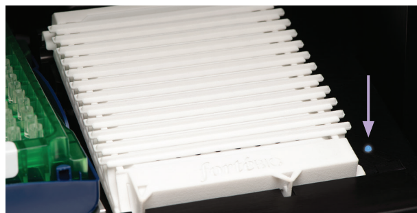
Figure 3: LED lights up when the evaporation cover is seated properly.
