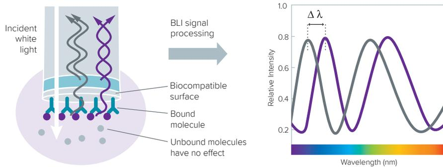
**Figure 3:** Bio-Layer Interferometry is an optical analytical technique that analyzes the interference pattern of white light reflected from two surfaces. Changes in the number of molecules bound to the biosensor causes a shift in the interference pattern that is measured in real time.
