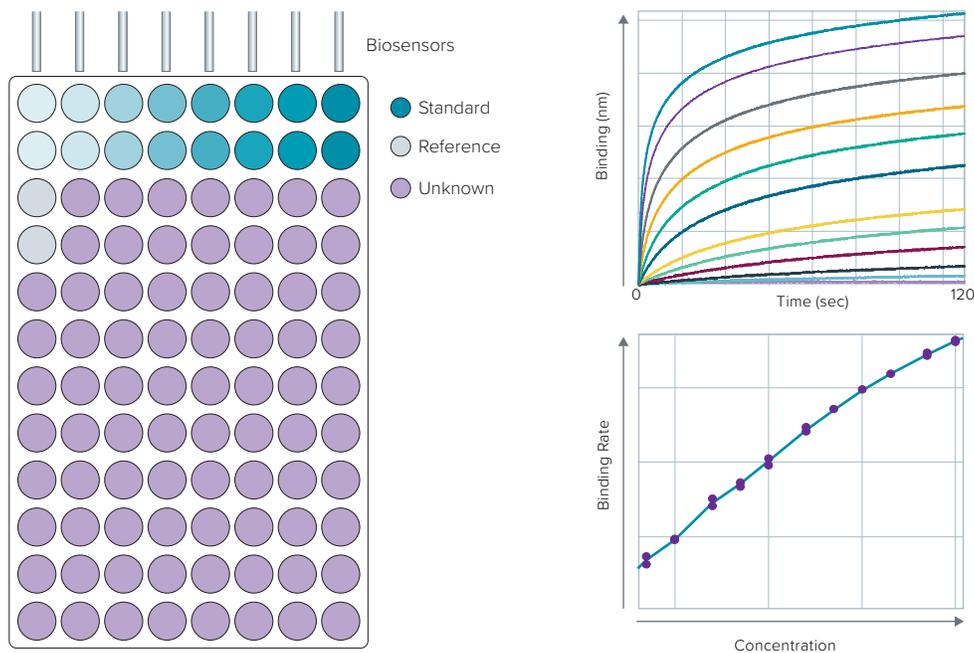
**Figure 4:** A typical quantitation assay setup. Biosensors dip into standards run in duplicate to obtain binding (nm shift) vs. time (sec) curves. The initial slope of the interaction is used to create the standard curve of the binding rate vs. concentration. The concentration of an unknown sample is then interpolated from the standard curve.
