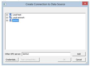
After selecting a server, you can optionally use the **Credentials**-button to specify a user, domain and password that you want to connect to the computer with. If not provided the account you are currently logged on as will be used for the configuration.
