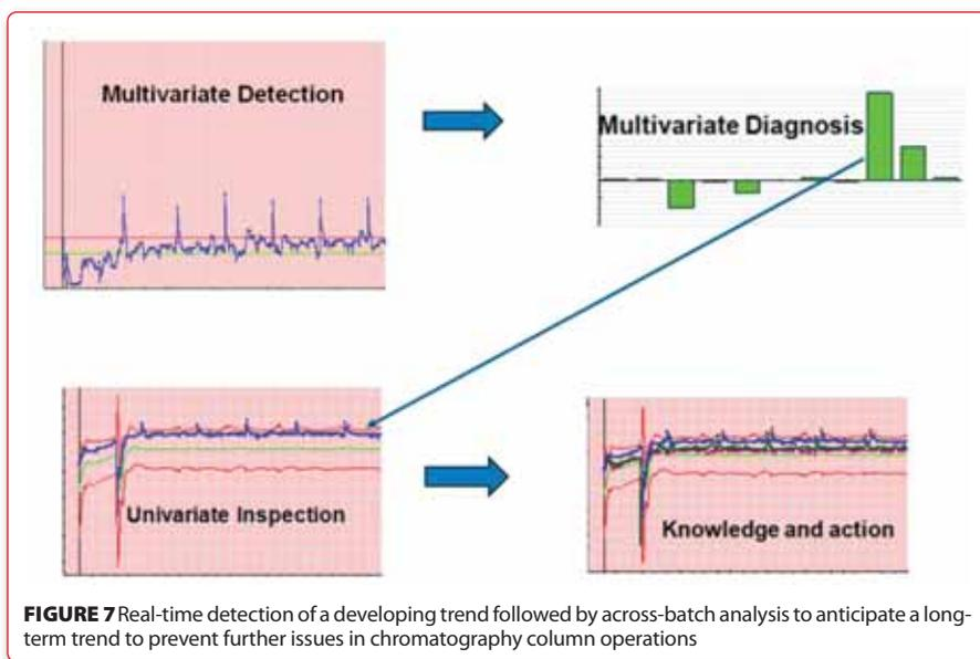
**FIGURE 7** Real-time detection of a developing trend followed by across-batch analysis to anticipate a long-term trend to prevent further issues in chromatography column operations
