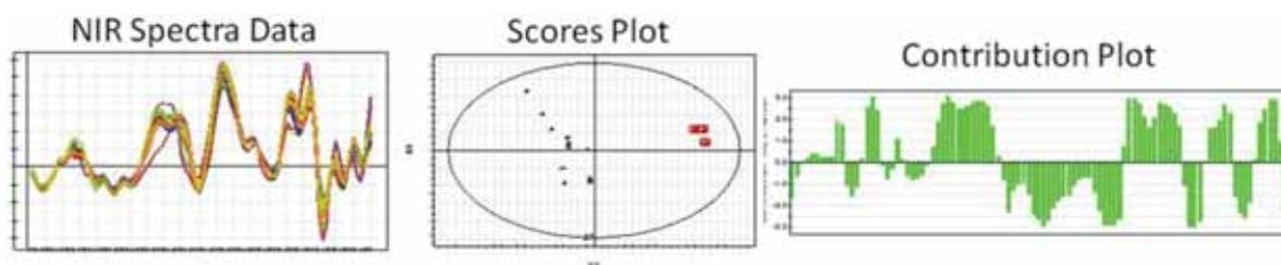
**FIGURE 4** Left – Processed NIR spectra data of different lots of the same raw material; Middle – Scores plot of a number of different lots of the same raw material; Right – Contribution plot of NIR spectra showing the differences of the raw materials lots highlighted in Red in the Scores plot vs. the rest of the lots
