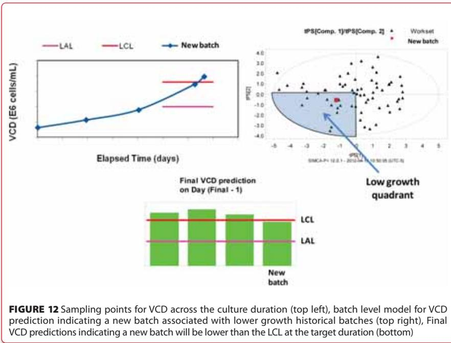
**FIGURE 12** Sampling points for VCD across the culture duration (top left), batch level model for VCD prediction indicating a new batch associated with lower growth historical batches (top right), Final VCD predictions indicating a new batch will be lower than the LCL at the target duration (bottom)
