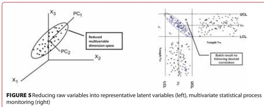
**FIGURE 5** Reducing raw variables into representative latent variables (left), multivariate statistical process monitoring (right)
