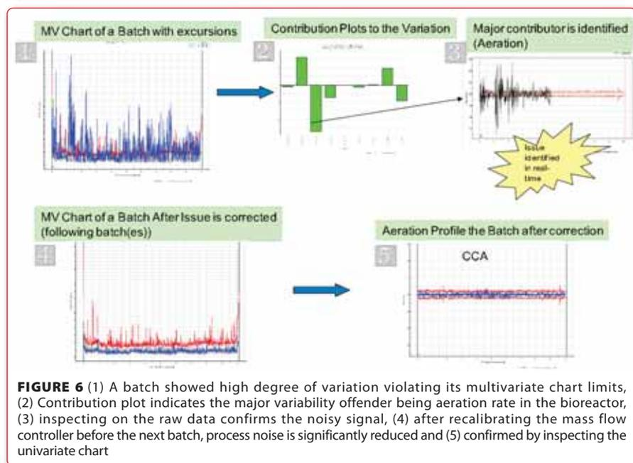
**FIGURE 6** (1) A batch showed high degree of variation violating its multivariate chart limits, (2) Contribution plot indicates the major variability offender being aeration rate in the bioreactor, (3) inspecting on the raw data confirms the noisy signal, (4) after recalibrating the mass flow controller before the next batch, process noise is significantly reduced and (5) confirmed by inspecting the univariate chart
