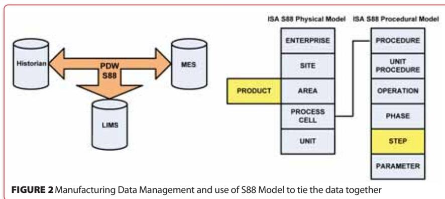
FIGURE 2 Manufacturing Data Management and use of S88 Model to tie the data together
