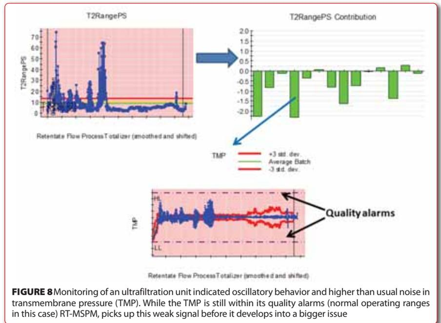
**FIGURE 8** Monitoring of an ultrafiltration unit indicated oscillatory behavior and higher than usual noise in transmembrane pressure (TMP). While the TMP is still within its quality alarms (normal operating ranges in this case) RT-MSPM, picks up this weak signal before it develops into a bigger issue
