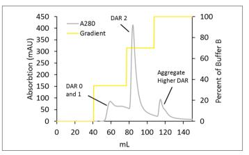
Figure 7: Small scale refinement of DAR distribution and aggregate removal. The crude reaction mixture was loaded to a Sartobind® Phenyl nano (3 mL), washed with 34% buffer B (25 mM sodium phosphate, pH 7.0, 20% (v/v) isopropyl alcohol), eluted using 70% buffer B, and finally stripped with 100% buffer B.
