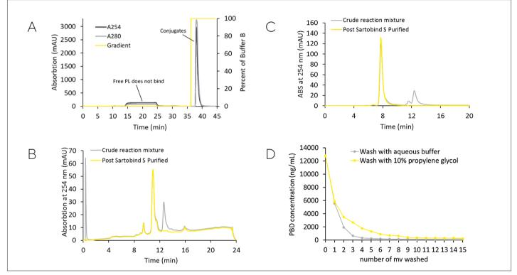
Figure 5: Removal of free payload by Sartobind<sup>®</sup> S at gram scale and analytical results (A). The quenched reaction mixture (gram scale) was loaded to a Sartobind<sup>®</sup> S 150 mL, then washed with 10 MV 20 mM MES pH 6.0 buffer prior to elution with 20 mM MES, 300 mM NaCl, pH 6.0 buffer. (B) HIC and (C) SEC profiles showing the removal of free PBD dimer. (D) Quantitative LC-MS data showing PBD dimer removal efficiency with Sartobind<sup>®</sup> S.
