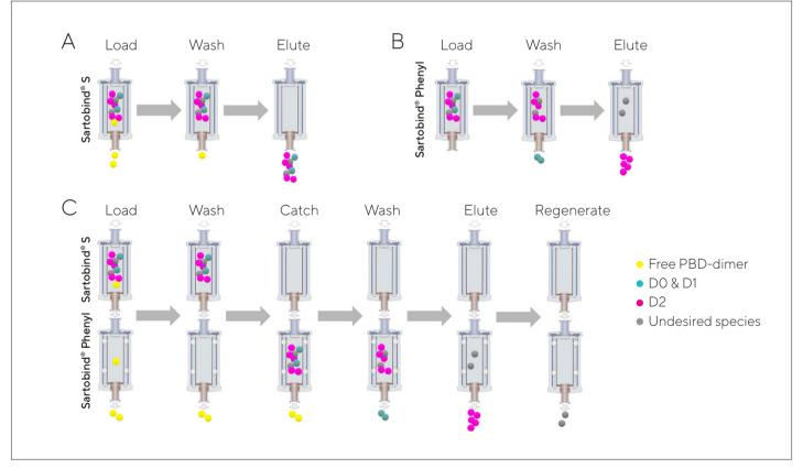
Figure 2: Sartobind<sup>®</sup> process overview. (A) Bind | Elute using Sartobind<sup>®</sup> S to remove residual payload, and (B) Bind | Elute using Sartobind<sup>®</sup> Phenyl to remove aggregate in stand-alone model; (C) Simplified process to purify target ADC with Sartobind<sup>®</sup> S and Phenyl in tandem model.
