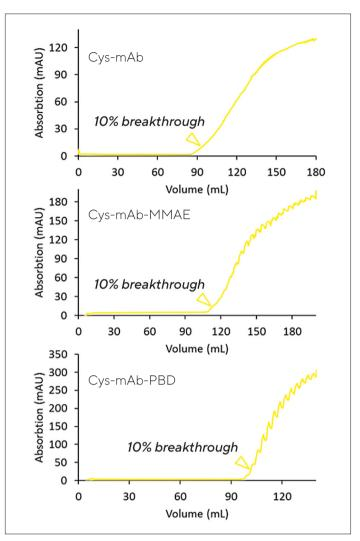
Figure 3: UV chromatograms at A280 for calculation of DBC at 10% breakthrough on Sartobind $^{\circ}$  S nano 3 mL.
