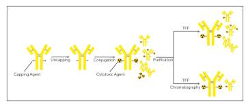
Figure 1: General method for manufacture of an engineered cysteine site specific ADC. Engineered cysteine antibody is diafiltered from the antibody formulation buffer into reduction reaction buffer, uncapped through reduction | oxidation steps, diafiltered into conjugation buffer, and conjugated to the cytotoxic agent, purified by chromatography (if necessary) and finally diafiltered into basal formulation buffer.
