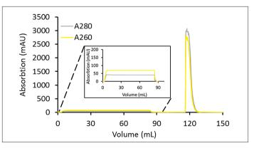
Figure 4: UV chromatogram at A280 for 82 mg load on Sartobind® S nano 3 mL.
