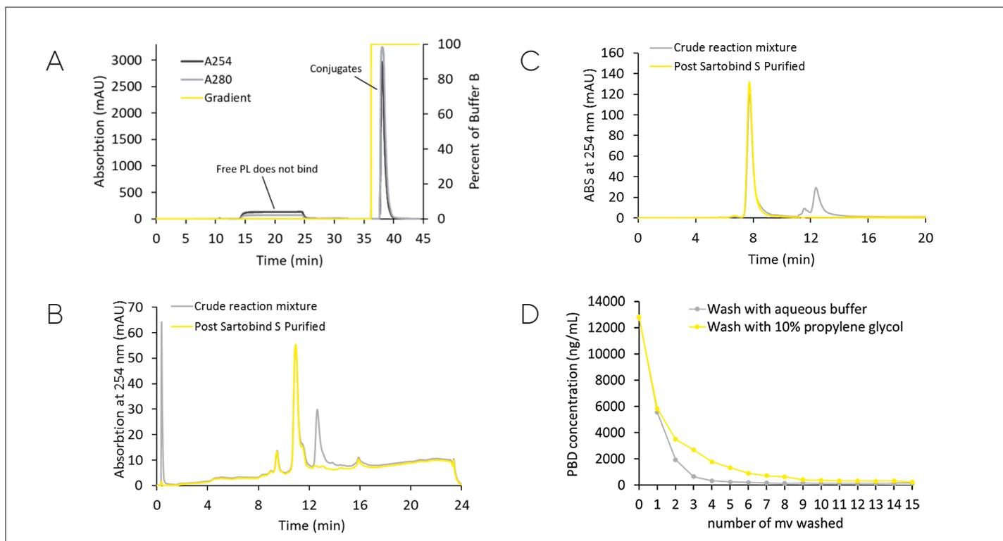
Figure 5: Removal of free payload by Sartobind® S at gram scale and analytical results (A). The quenched reaction mixture (gram scale) was loaded to a Sartobind® S 150 mL, then washed with 10 MV 20 mM MES pH 6.0 buffer prior to elution with 20 mM MES, 300 mM NaCl, pH 6.0 buffer. (B) HIC and (C) SEC profiles showing the removal of free PBD dimer. (D) Quantitative LC-MS data showing PBD dimer removal efficiency with Sartobind® S.
