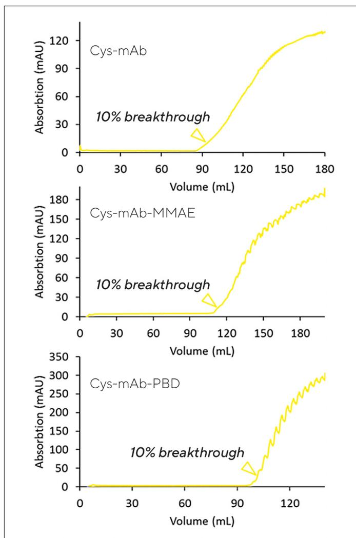
Figure 3: UV chromatograms at A280 for calculation of DBC at 10% breakthrough on Sartobind® S nano 3 mL.
