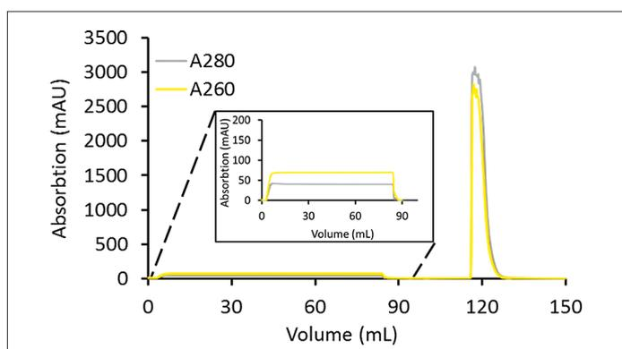
Figure 4: UV chromatogram at A280 for 82 mg load on Sartobind® S nano 3 mL.
