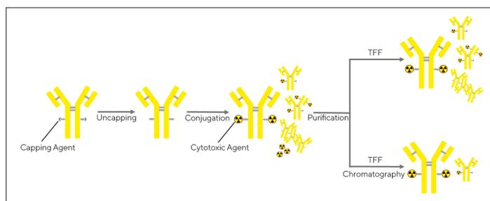
Figure 1: General method for manufacture of an engineered cysteine site specific ADC. Engineered cysteine antibody is diafiltered from the antibody formulation buffer into reduction reaction buffer, uncapped through reduction | oxidation steps, diafiltered into conjugation buffer, and conjugated to the cytotoxic agent, purified by chromatography (if necessary) and finally diafiltered into basal formulation buffer.
