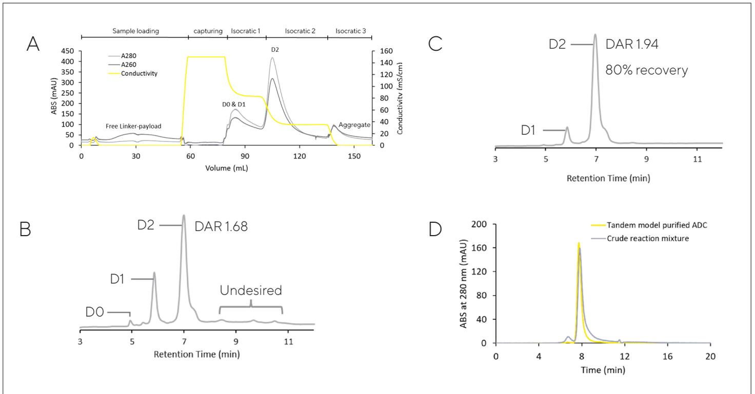
Figure 9: Free payload removal, aggregate removal and DAR distribution refinement in a single unit operation. (A) A total of 30 mg crude conjugate mixture was loaded on a 3 mL Sartobind® S and a 3 mL Phenyl membrane were used in tandem (series). (B) HIC HPLC chromatogram of load. (C) HIC HPLC chromatogram of the second isocratic elution. (D) SEC HPLC chromatogram of the second isocratic elution.
