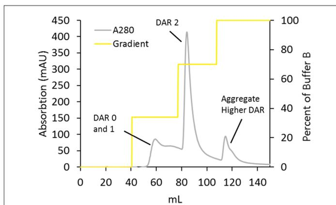
Figure 7: Small scale refinement of DAR distribution and aggregate removal. The crude reaction mixture was loaded to a Sartobind® Phenyl nano (3 mL), washed with 34% buffer B (25 mM sodium phosphate, pH 7.0, 20% (v/v) isopropyl alcohol), eluted using 70% buffer B, and finally stripped with 100% buffer B.
