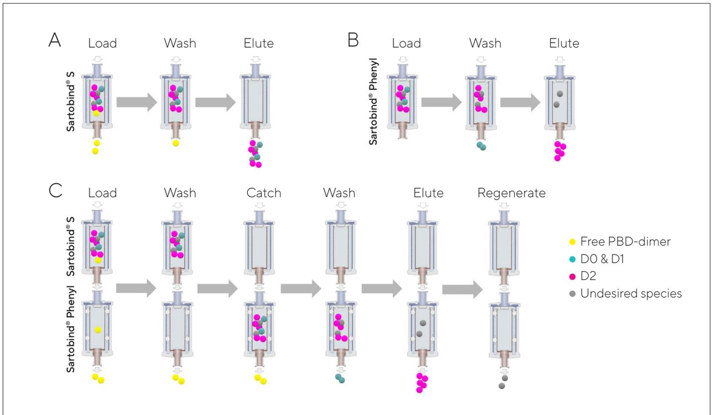
Figure 2: Sartobind® process overview. (A) Bind | Elute using Sartobind® S to remove residual payload, and (B) Bind | Elute using Sartobind® Phenyl to remove aggregate in stand-alone model; (C) Simplified process to purify target ADC with Sartobind® S and Phenyl in tandem model.
