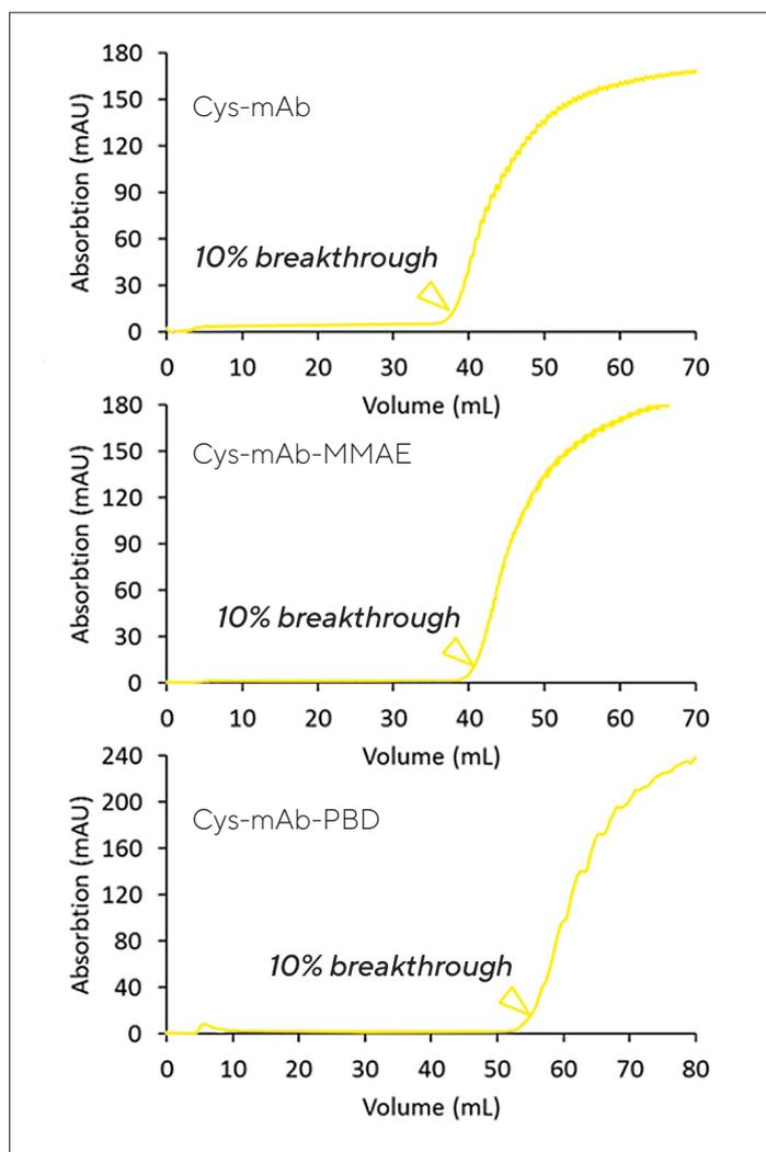
Figure 6: UV chromatograms at A280 for calculation of DBC at 10% breakthrough on Sartobind® Phenyl nano 3 mL.
