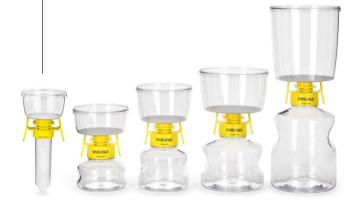
Clarification and sterile filtration are performed in a single step, which enables cell cultures to be efficiently clarified and sterilized in minutes.
