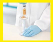
4. One minute later, the clarified cell culture liquid is available for subsequent downstream processing steps, such as protein purification and concentration.
