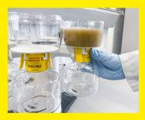
4. Rotate the head of the Multistation and filter the next samples or remove the filtration unit after filtration.
