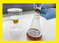
2. Mix to homogenize. Pour the cell culture and filter aid mixture into the Sartolab® RF first, ...
