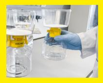
2. Pour the cell culture and filter aid mixture into the Sartolab® RF filtration unit.
