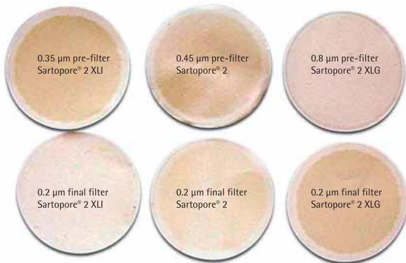
Fig. 1: 47 mm filter discs of Sartopore® 2 XLI, Sartopore® 2 and Sartopore® 2 XLG after filtration of Glucose solution
