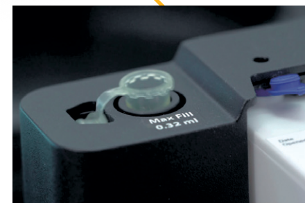
Onboard vortexing just prior to sampling ensures proper resuspension and delivers improved QC results and consistency.
