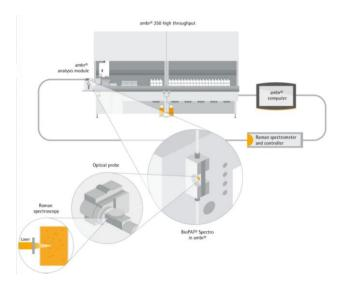
Caption: BioPAT® Spectro, a Quality by Design (QbD) tool for use with ambr® automated micro and mini bioreactor systems to enable Raman spectroscopy capability. Schematic showing the technology in use with ambr® 250 high throughput
