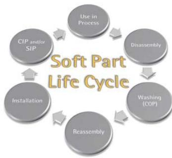
Assemblies that include soft parts are typically removed from process equipment, disassembled, and cleaned out of place (COP) before being reassembled for reuse. The maintenance of multi-use stainless steel parts should be closely monitored during its lifetime to preserve the thin passive oxide layer which is intrinsic to the surface when new (Cluett, 2001). Corrosion or breakdown of this ultra-thin layer, be it chemical or
