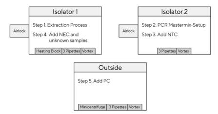
It is also possible to connect Isolator 1 and Isolator 2 via an airlock so that you can transfer the PCR tubes after Step 3 directly from Isolator 2 into Isolator 1.
