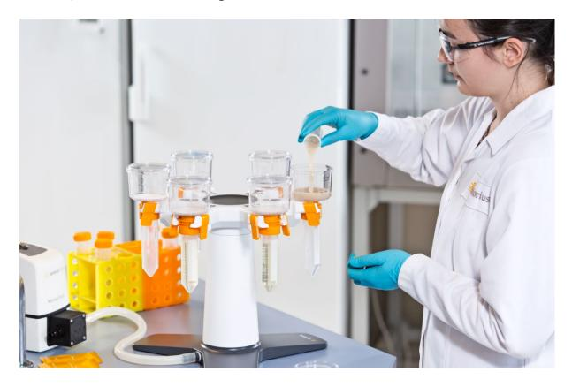
**Sartolab® MultiStation –** A stand with one vacuum connection, a rotating, multi-directional head and 6 brackets for hands-free parallel filtration of up to 6 x 50 mL samples
