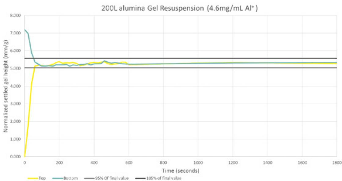
Fig.4:Alumina gel resuspended in less than a minute at a low speed of 150 rpm in 200 L Flexsafe® Bag for Pro Mixer
