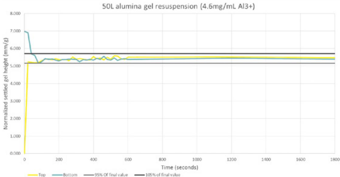
Fig. 3: Alumina gel resuspended in less than a minute at a low speed of 115 rpm in 50 L Flexsafe® Bag for Pro Mixer
