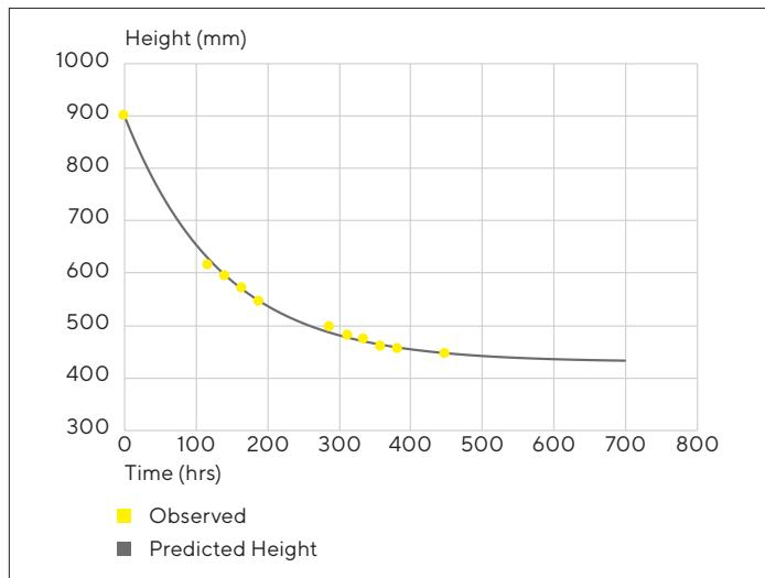
Fig 1: Alumina gel cloud height versus settling time
