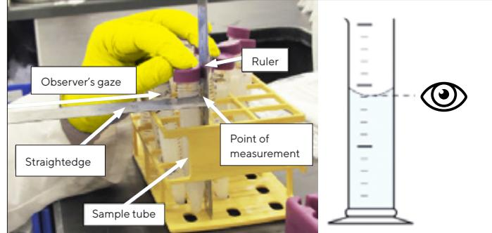
Use a ruler to determine settled gel height. It can be helpful to use a straightedge oriented parallel to the observer's gaze as a measurement aid.
