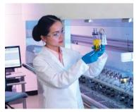
ambr<sup>®</sup> 250 is a fully automated bioreactor system offering independent, parallel control of 12 or 24 single-use bioreactors
