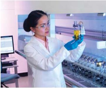
ambr® 250 is a fully automated bioreactor system offering independent, parallel control of 12 or 24 single-use bioreactors
