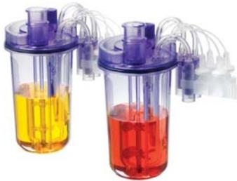
ambr 250's easy connect bioreactors are fully integrated with sensors and filters
