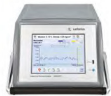
LMA321 At-line moisture analyzer for measuring the moisture and density of pourable and granular products, such as ground coffee or grain, in fractions of a second in laboratories or next to production lines
