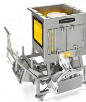
Flexel® Palletank® System Container for mixing, transportation and storage of biopharmaceutical culture media in sterile Flexel® 3D single-use bags
