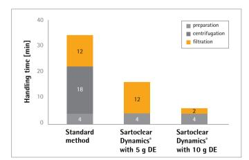
Figure 2: Comparison of clarification methods by handling time. Sartoclear Dynamics<sup>®</sup> Lab significantly reduces the amount of time required to clarify cell culture media.
