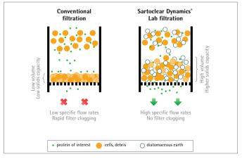
Figure 1: Principles of clarifying cell cultures by using the conventional and the body-feed-filtration method utilised by Sartoclear Dynamics<sup>®</sup> Lab
