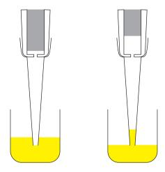
How an air displacement pipette works
