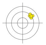
Result is accurate and precise: The mean volume equals the set volume; there is only minor variation between pipetting results.
