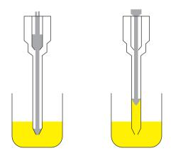
How a positive displacement pipette works
