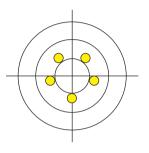
Result is precise, but not accurate: There is only minor variation between pipetting results; however, the mean volume differs from the set volume.
