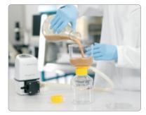
2. Mix to homogenize. Pour the cell culture and filter aid mixture into the Sartolab<sup>®</sup> RF first, ...
