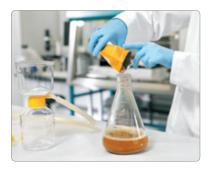
1. Attach the Sartolab<sup>®</sup> RF unit to a vacuum source. Pour the filter aid into your cell culture.
