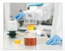
3. ... then filter by simply using the pump.
