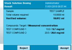
YAPP16 checks and verifies the weight of compounds during preparation of standards.
