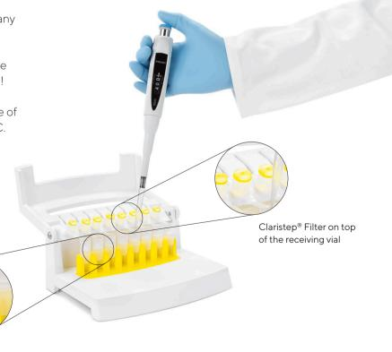
Receiving vial positioned in the Claristep® Station tray
