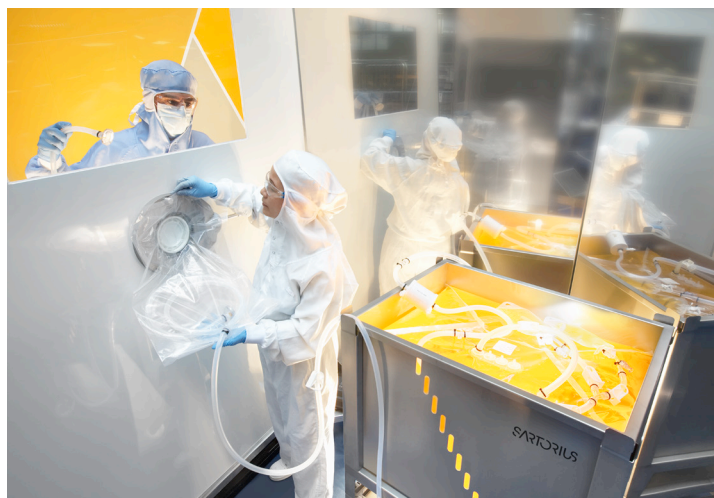
Figure 1: Zone-to-zone liquid transfer using the Biosafe® Rapid Transfer Port
