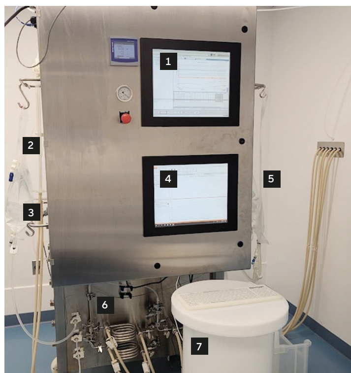
Figure 1: DIANT® PILOT with single-pass TFF and Sartorius Products. All-in-One Skid to Produce and Concentrate Nanoparticles
