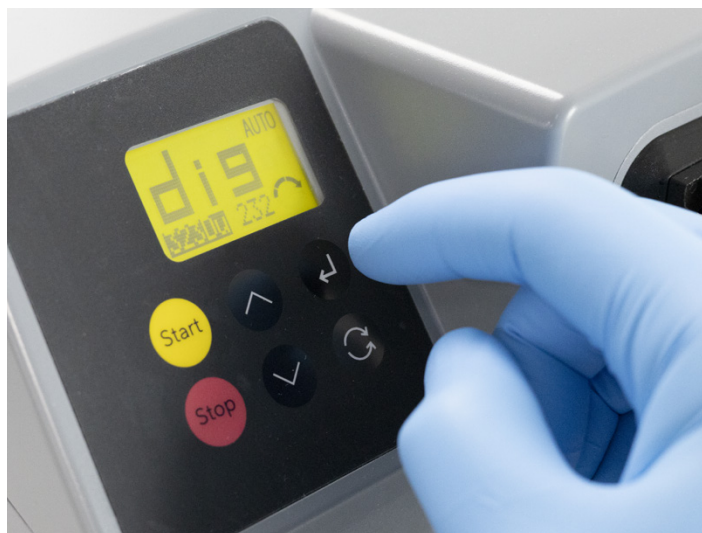
Figure 5: Pump display showing the pump in digital mode.
