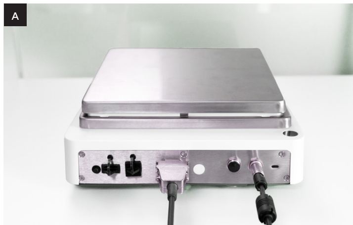
Figure 4: RS232 data cable connection to the balance (A) and pump (B).
