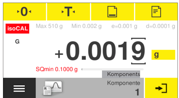
Figure 5: Display of a Secura524-1S with switched on SQmin function. If the value that has been determined based on the USP and stored by Sartorius Service of, in this case, 0.1 g is not reached, the indication of the minimum sample weight lights up in red. With a correspondingly set higher security level, the weighing result is also identified as "not valid" by the exclamation mark and | or the result cannot be expressed or printed..
