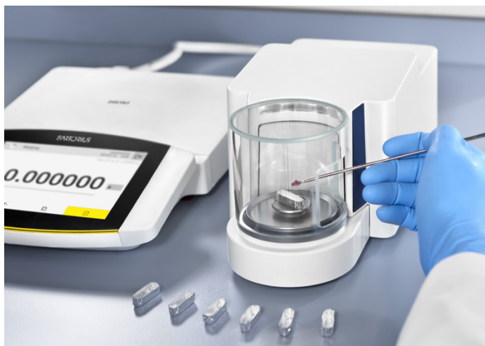
Figure 1: Weighing smallest amount of substance on a microbalance
