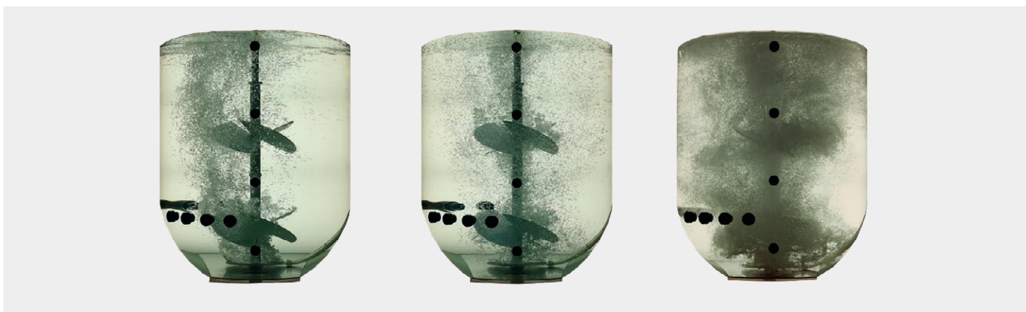
Figure 10: Images Showing Transition From Heterogeneous to Homogeneous Gas Distribution in the Biostat STR ® 2,000 L. 0.3 m/s Tip Speed With 0.05 vvm Aeration (Left), 1.2 m/s Tip Speed With 0.025 vvm (Center), and 1.8 m/s Tip Speed With 0.1 vvm
