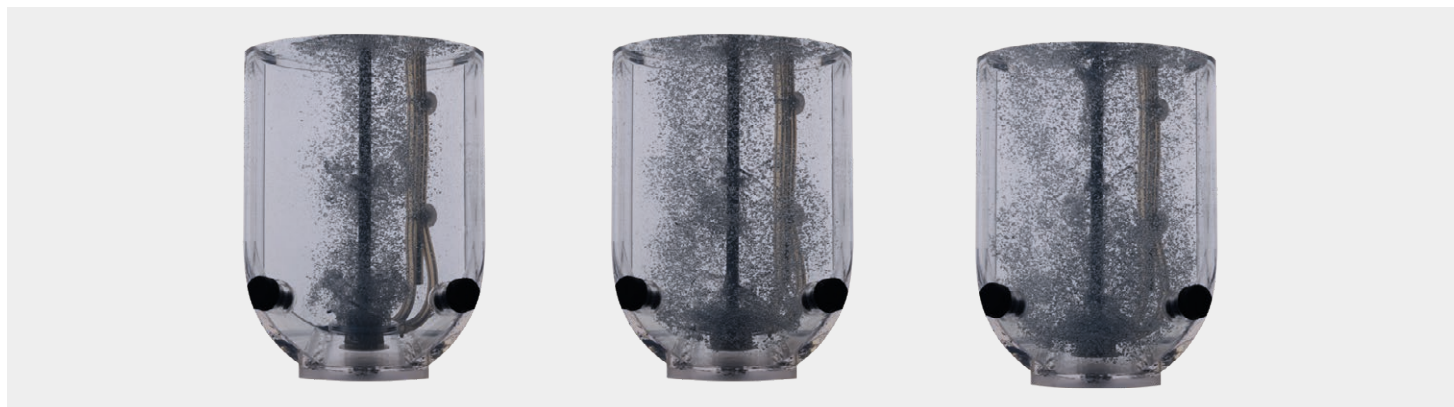
Figure 9: Images Showing the Transition From Heterogeneous to Homogeneous Gas Distribution in the Biostat STR ® 50 L. Two-Segment Impeller With 0.1 vvm Gassing Rate at 0.6 m/s (Left), 1.2 m/s (Center) and 1.8 m/s Tip Speed (Right)
