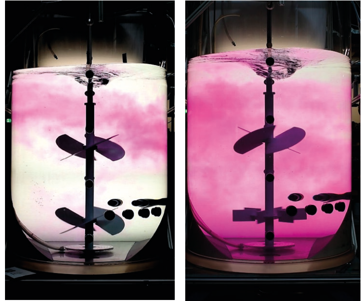
Figure 2: Images of Decolorization Progress in the Biostat STR® 2,000 L After 23 Seconds With Two-Segment Impellers (Left) and With More Dye Residues Below the Rushton Stirrer (Right)
