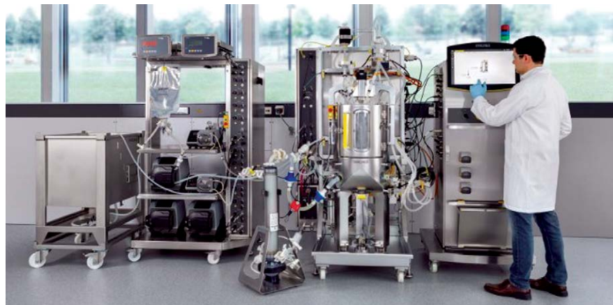
Sartorius Biostat STR with alternating tagential-flow (ATF) filtration system
