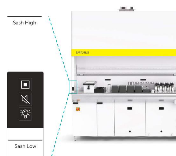
Figure 10: An ergonomic keypad is positioned on the frame for quick system interactions
