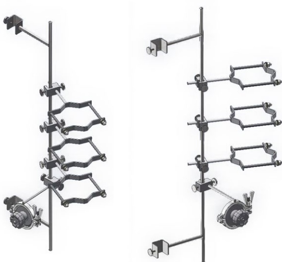
Figure 2: CAD Drawing of the Hollow Fiber Mounting Brackets
