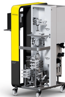
Figure 4: Resolute® BioSC Configured for Rapid Cycling Chromatography
