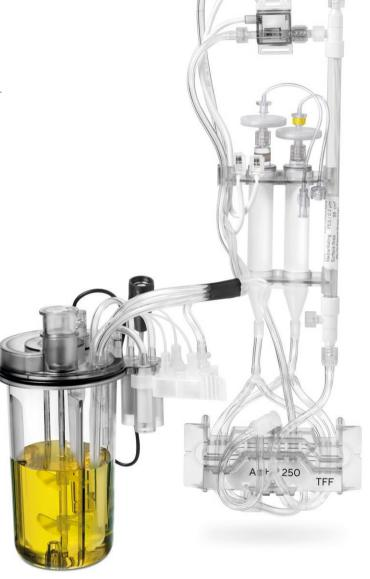
Ambr<sup>®</sup> 250 High Throughput perfusion TFF vessel with 0.2 µm filter
