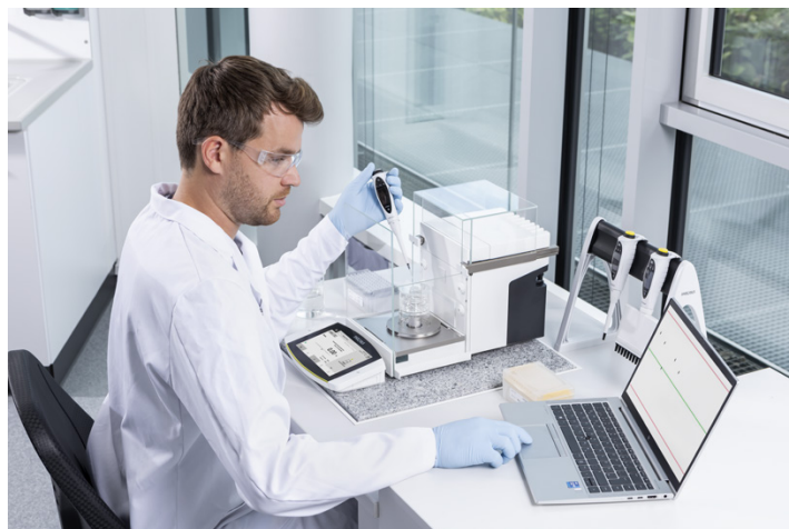
Figure 1: Picus® 2 Electronic Pipette Calibration with Cubis® II Balance, Evaporation Trap and Ingenix Software
