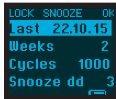
Information when the last calibration has been made
