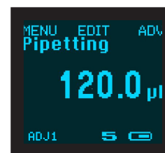
The pipette is set to use the adjustment values saved to ADJ1.
