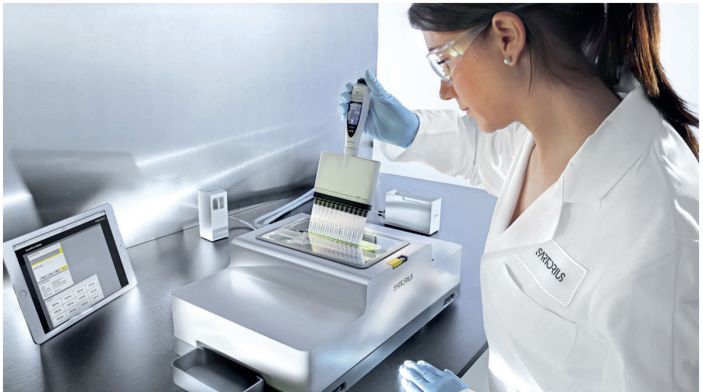
Figure 2: Gravimetric Calibration on a Speedcal Mobile Multi Channel Balance
