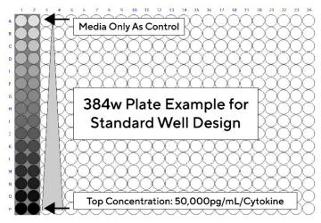
Figure 6. Recommended 384-well plate layout
