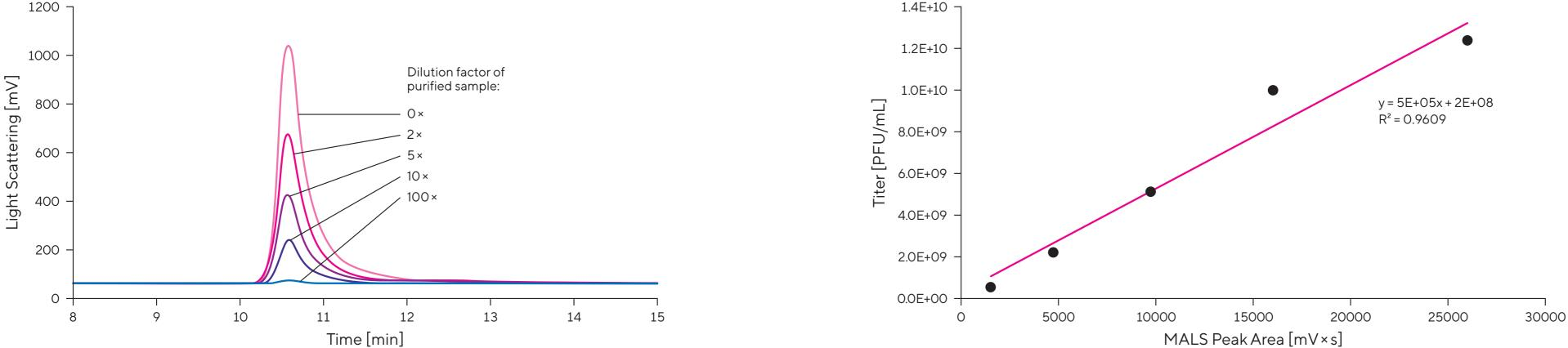
Figure 1: Illustrates a Calibration Curve Generated From a Dilution Series of Purified Phage (T4) And Measured by MALS. The Figure Also Illustrates Values Obtained by Measuring Each of the Dilutions by Plaque Assay (Values in Black).
