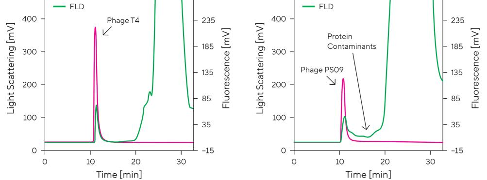
Figure 3: Illustrates the Size Exclusion Chromatography Profile of a Phage-Containing Clarified Cell Culture Harvest of Two Different Phages, Monitored by Fluorescence (FLD) And Multi-Angle Light Scattering (MALS): Harvest of Bacteriophage T4 (Left) And Harvest of Bacteriophage PSO9 (Right).
