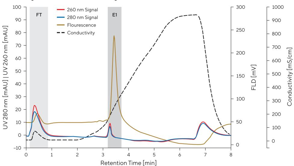
Figure 2: Chromatogram for Influenza A Virus Separation on CIMac SO3-0.1 Analytical Column
