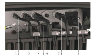
1 Earth 2 Future environmental, temperature sensor 3 External pressure sensor 4 External valves
