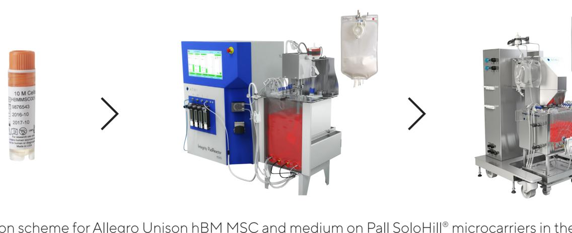
Expansion scheme for Allegro Unison hBM MSC and medium on Pall SoloHill® microcarriers in the Allegro Microcarrier Delivery System (AMDS) using Pall's PadReactor System. Cells thawed from liquid nitrogen were seeded directly onto collagen microcarriers in the PadReactor Mini bioreactor at 6 L and expanded for 3 days. Cells were harvested and seeded onto collagen microcarriers (AMDS) in the PadReactor 50 system at 40 L and cultured for 5 days.
