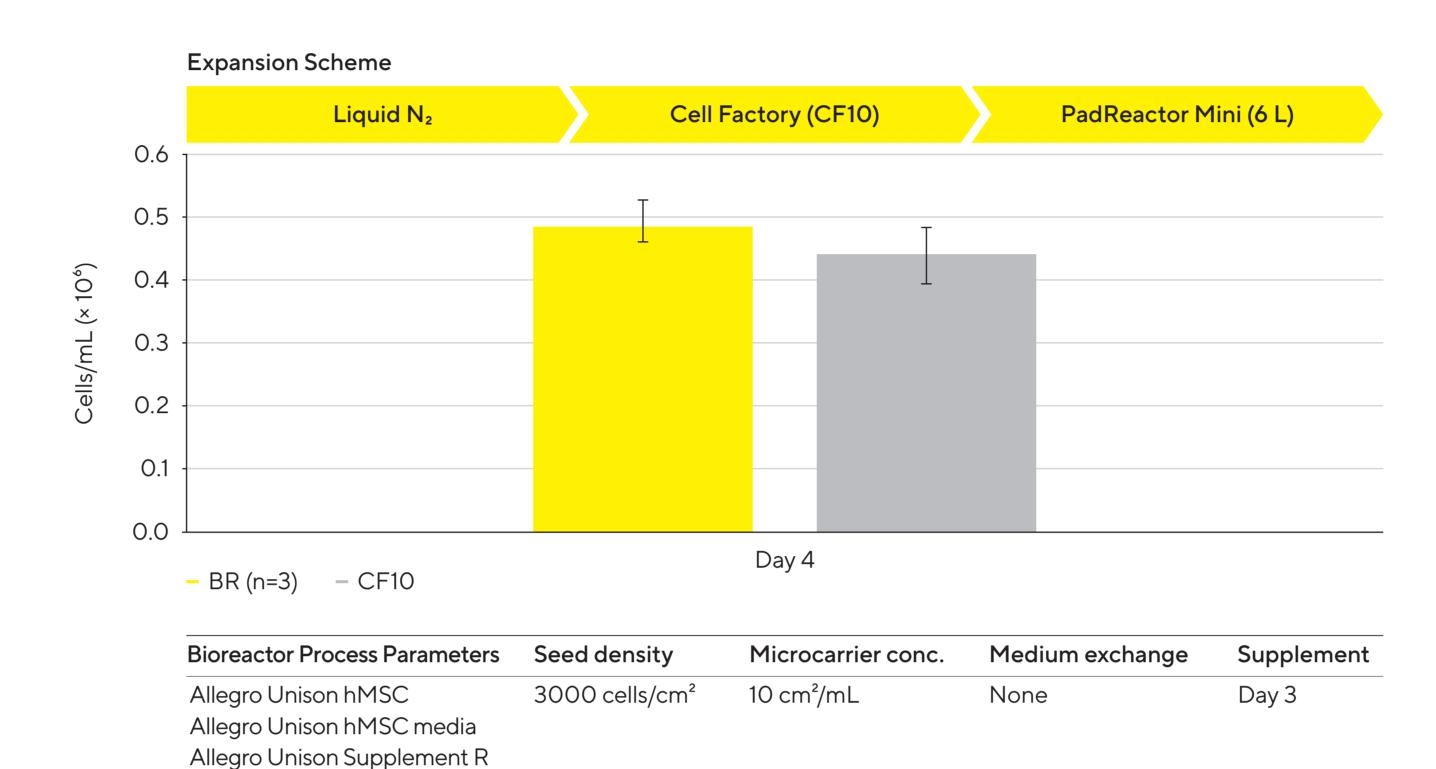
Reproducible expansion of hMSC on SoloHill<sup>®</sup> microcarriers in PadReactor bioreactors. Cell densities reached approximately 0.5 million cells per mL and over twenty-fold expansion was reproducibly achieved in fed-batch microcarrier cultures in the PadReactor Mini bioreactor at 6 L scale in 4 days (BR n = 3).
