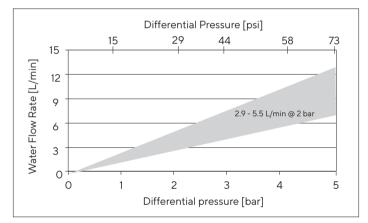
The water flow rate for the Virosart<sup>®</sup> Media mid-scale modules 0.3 m<sup>2</sup> is 420 LMH/bar ±30%, 25 °C.
