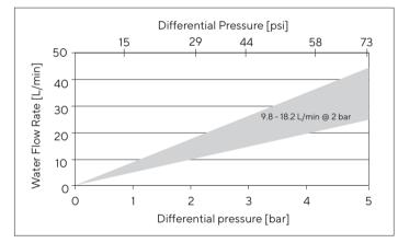
The water flow rate for the Virosart® Media process modules 1.0 m<sup>2</sup> is 420 LMH/bar ±30%, 25 °C.
