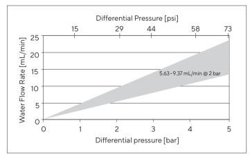
Due to the shorter fiber length in the Virosart $^{\circ}$  Media lab module, the water flow rate is 450 LMH/bar ±25%, 25 °C.
