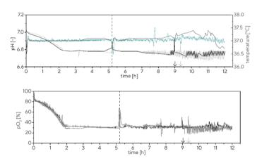
**Figure 3:** Process control of both cultivations. The pO<sub>2</sub>, was controlled by changing the tip speed and supplementing oxygen (fig. 1). Additionally, pH and temperature were also controlled. Biostat<sup>®</sup> B-DCU data were colored and data from a former cultivation were light-colored, respectively.
