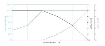
Figure 1: Schematic  $pO_2$  cascade of both cultivations. Starting with a constant air gas flow of 5 lpm,  $pO_2$  was controlled by increasing tip speed to 1500 rpm and supplementing oxygen.
